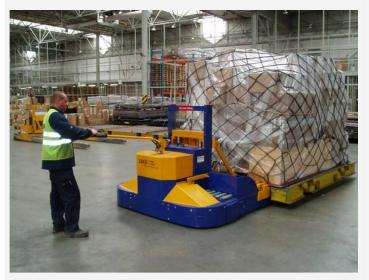
Our safe and cost effective system for flexible handling of air cargo on slave pallets. By using the purpose designed Pallet Master, slave pallets can be docked with fixed conveyor systems at standard 508 mm / 20 inch dolly height for transfer of ULD's loaded up to 6800 kg. 10ft ULD's can be built or broken at any place in the warehouse so that you are no longer limited to the use of fixed work stations.
